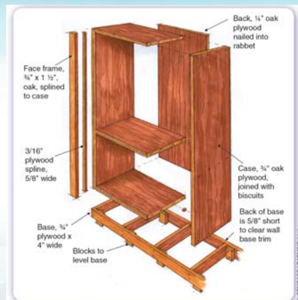
Figure 8-24: An example of a technical drawing that is used to describe the main details of a project. This particular drawing is hand-drawn and is "exploded" to show the construction and assembly details. The drawing also contains annotations that provide additional information.
